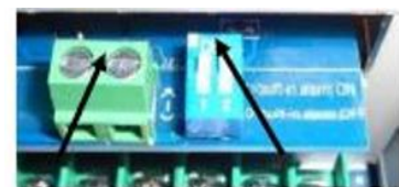
Terminal strip J22 Toggle switches
